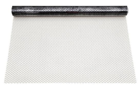
ESD Grid PVC curtain is made of transparent PVC material with permanent antistatic agent; if black grid curtain is mad with black conductive oil ink printing on transparent PVC film, and make its grid side with better antistatic property.
